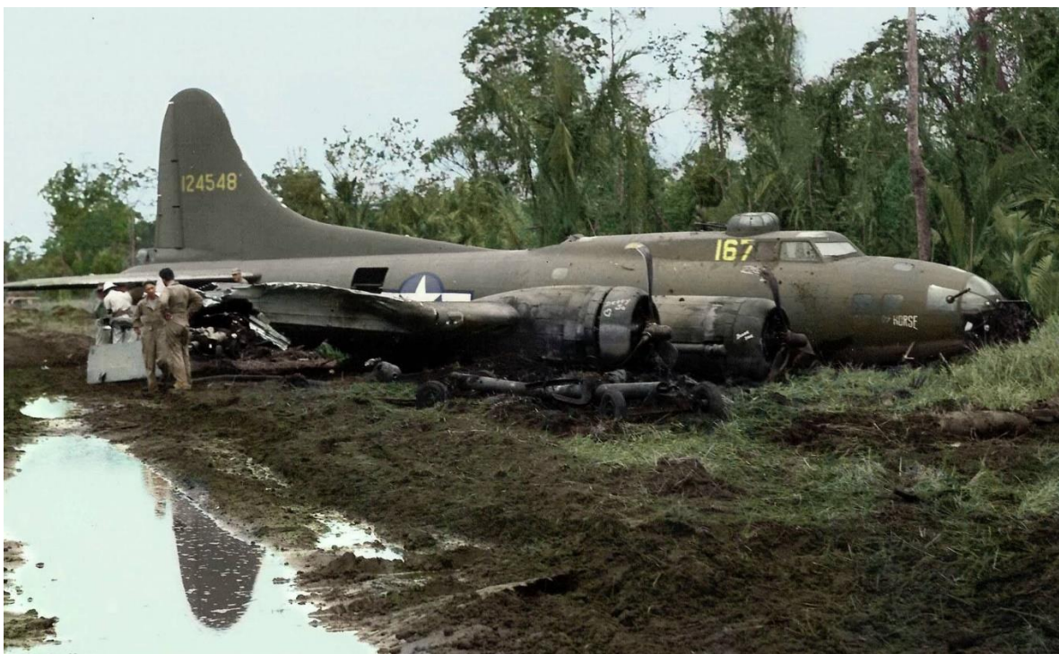
375 TCG B-17 that crashed at Nadzab after a supply airdrop mission over Hollandia, May 1944. The aircraft ran out of fuel and the right wheel collapsed upon landing, sending the plane off the runway.
