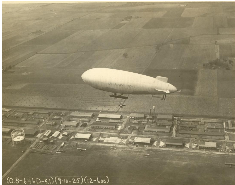
The hookup of the Sperry Messenger with the TC-7 in 1925. Note the circular frame on the left, which supported an expandable bladder as part of the helium storage and repurification plant.
